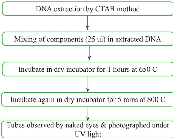
**Figure 1 Flow chart of LAMP-HNB based for HLB detection**
